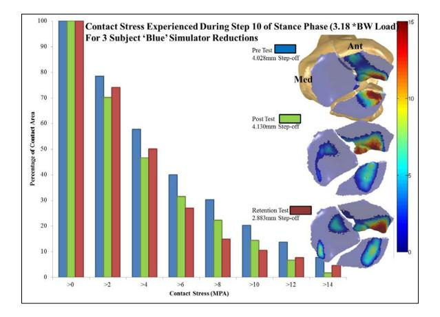
Figure 17: Contact stress experienced during step 10 of stance phase for subject Blue simulator trials. Contact Area illustrated on right.
