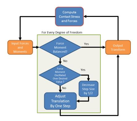
Figure 8: Flowchart of iterative load control system which manipulates translations and rotations to push the DEA algorithm to equilibrium.
