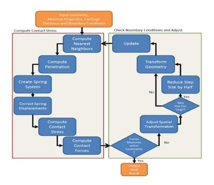
Figure 7: Flowchart of DEA algorithm where subject-specific geometries, material properties, cartilage thicknesses and boundary conditions are input into the algorithm.
