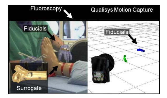
Figure 3: The tibial plafond simulation in the earliest form. Single camera feed shown on left with view of hand motion and fluoroscopic monitor. Qualisys motion capture software displaying the synced motion capture data with each hand's fiducial markers. In lower left, a fracture constellation is shown from the lateral view of the lower left leg.
