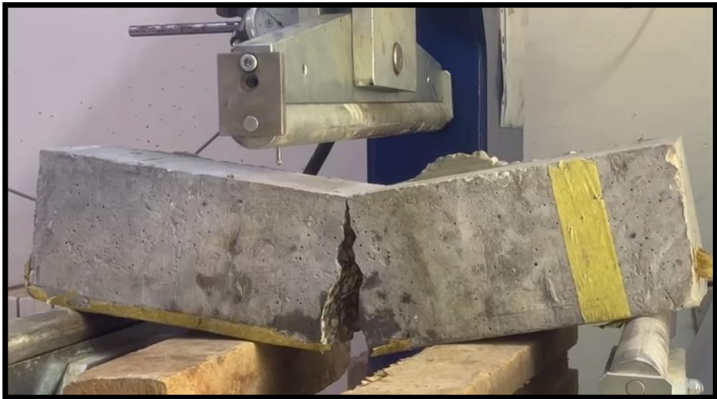
Figure 4.24: Depicts the Failure Behavior of a Plain Concrete Specimen (Control Specimen)
