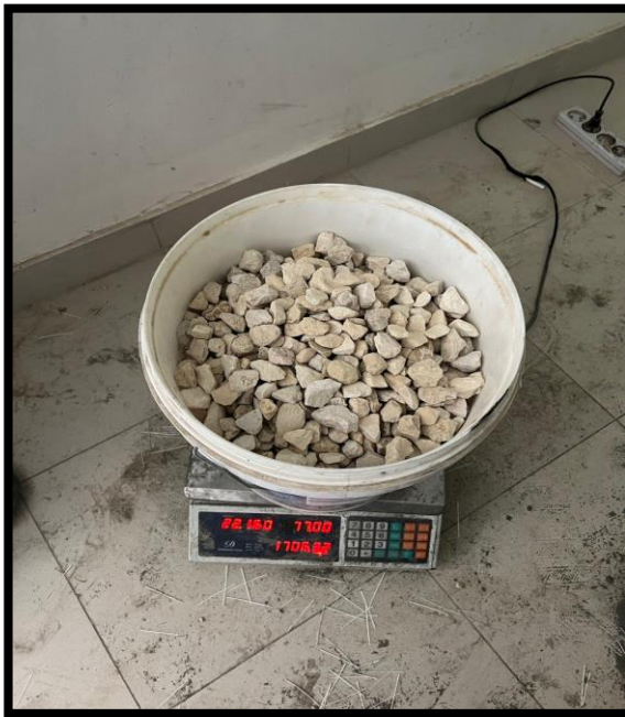
Figure 3.3: Signifies the Exact Preparation of the Concrete Mix, Requiring Precise Measurements of Cement, Aggregate, Water, and any Related Chemical Additives.
