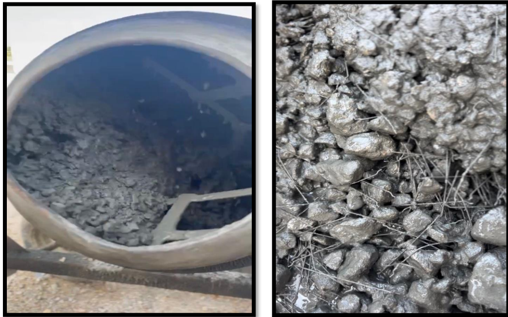
Figure 3.4: A Concrete Mixer Ensured Consistent and Uniform Blending of Components, with a Specific type and Amount of Fiber Evenly Distributed Throughout the Mixture.
