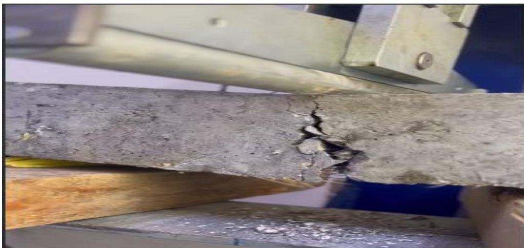
Figure 4.25: Illustrates the Response of Fiber-Reinforced Concrete Specimens.
