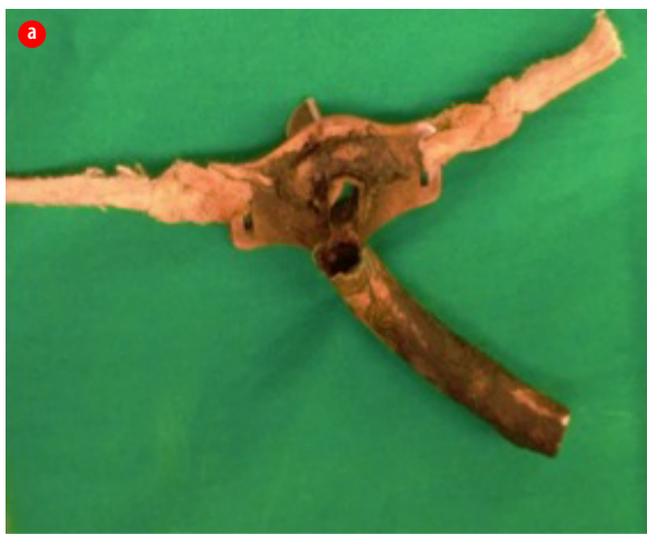
Figure 2: Photographs showing the (a) broken inner tube of the metallic tracheostomy tube, and (b) the broken inner segment of the tube.
